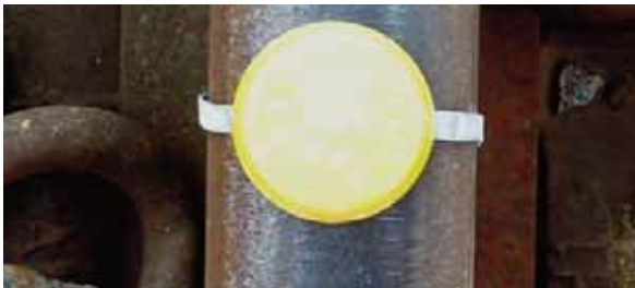
Detonator secured to rail
